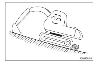
Avoid traveling in a cross direction on a slope as it can cause the danger of rolling over and sliding.
